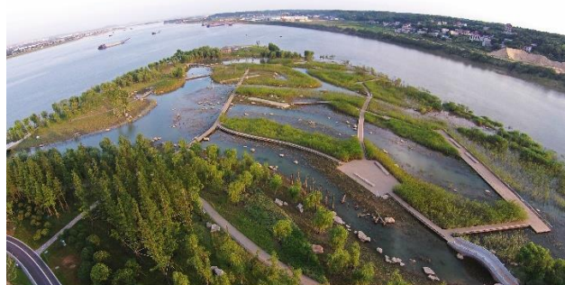
Variable grading makes the flood fluctuation no longer a threat, offering instead an opportunity for increasing biodiversity. Different water levels contribute to various habitats. This image shows the south wetland in summer with high water level.
